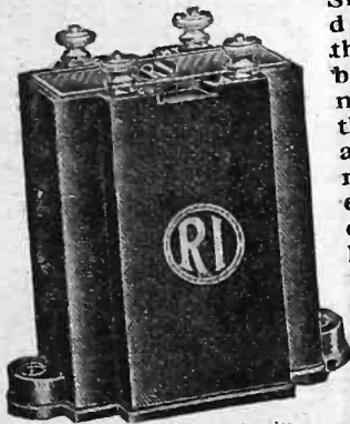
Inductance primary 85 henries. Resistance primary D.C. 1,400 ohms. Resistance secondary D.C. 8,000 ohms. Ratio 4 to 1.
